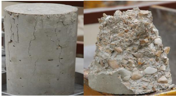
**Figure 6: Compressive strength test. (a) Appearance of cracks in the lateral surfaces of the test specimen due to tensile stresses; (b): Conical rupture of the specimen**
