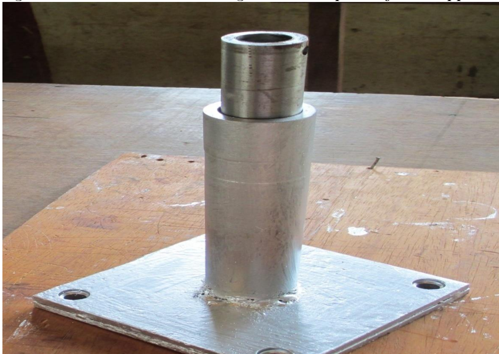
Plate 1 Briquette Compression Cylinder and the Piston (Fabricated)
