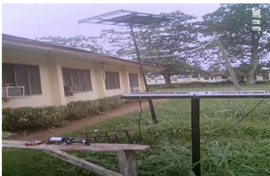
Figure 1a: The Prototype of Solar Array of Test ASPS
