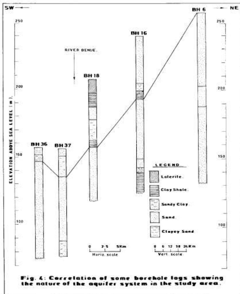
Fig. 4: Correlation of some borehole logs showing the nature of the aquifer system in the study area.
