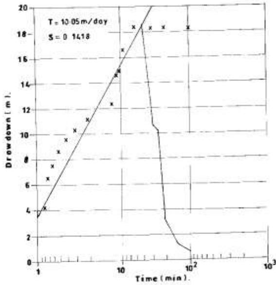
**Fig. 6: Relation between time and drawdown for aquifer test of well BH 13.**
