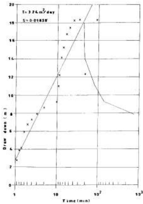
**Fig.7 Relation between time and drawdown for aquifer test of well BH 37**
