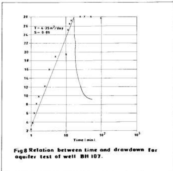
Fig 8 Relation between time and drawdown for aquifer test of well BH 107.
