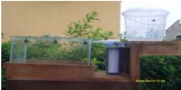
Fig 1.1: Constructed 12watt UV purifier with a 12v, 100AH battery
