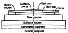
Although a pavement's wearing course is most prominent, the success or failure of a pavement is more often than not dependent upon the underlying sub grade - the material upon which the pavement structure is built [9]. Sub grades can be made of a wide range of materials although some are much better than others. It is stated in [7] that a sub grade's performance generally depends on three of its basic characteristics (all of which are interrelated):
