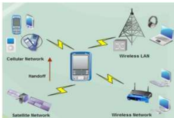
Figure 3: Accessing multiple networks and services through multi-mode software
