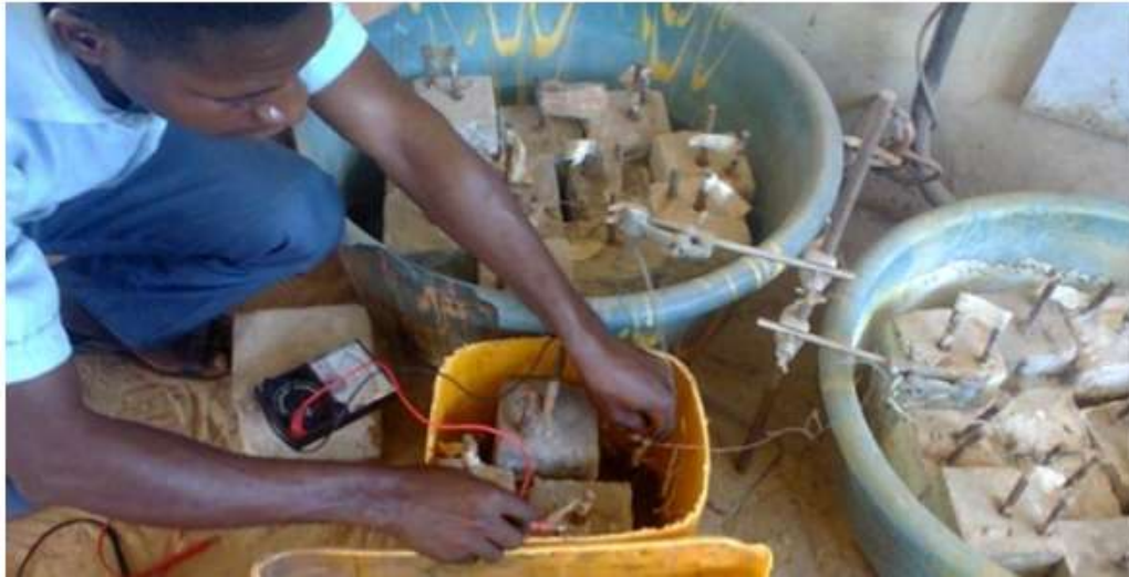
Figure 4. Picture showing Corrosion Readings been taken from Concrete Samples
