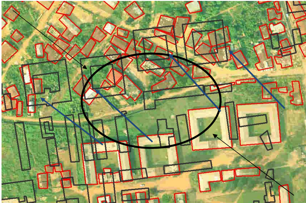
Fig. 3.4: GIS error resulting from variations in original data sets (Black-digitised from Google Earth Imagery and the Red-digitised from Orthophoto)
