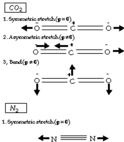
Figure-10: Normal vibrational modes of CO<sub>2</sub> and N<sub>2</sub>
