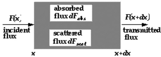
Figure-17: Transmission of radiation through an elemental slab
