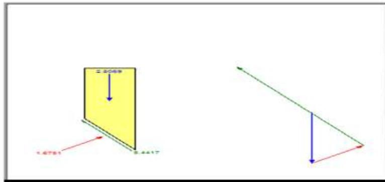
Figure 11b: Force Polygon on the Critical Slice Mass
