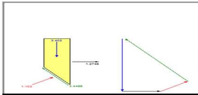
Figure 10b: Force Polygon on the Critical Slice Mass
