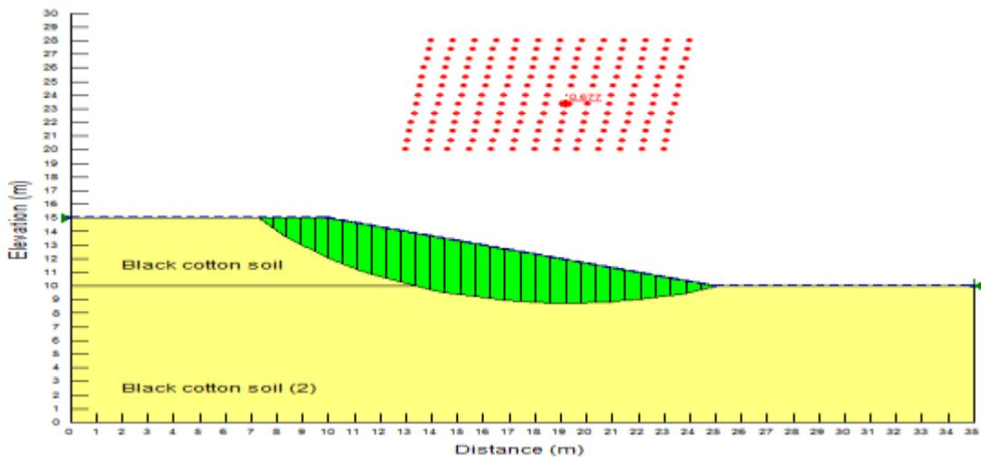
Figure 11a: Graphical View of the Computed Detail for Fully Saturated Slope
