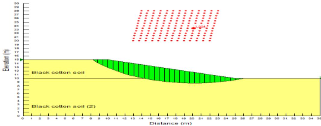
Figure 10a: Graphical View of the Computed Detail for Dry Slope
