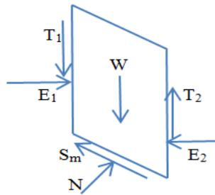
Figure3: Forces Acting on a Slice in BSM.
