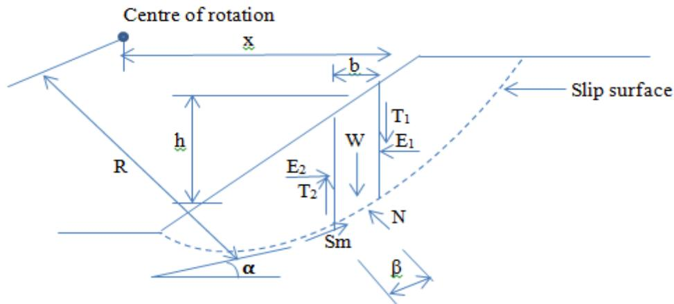
Figure 1: Circular Slip Surface with Underlying Soil Mass Divided Into Vertical Slice (Fredlund & Rahardjo, 1993)
