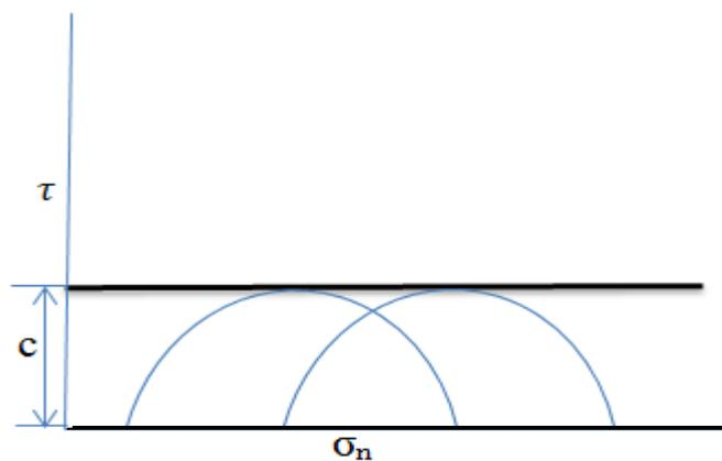
Figure 8: Undrained Strength Envelope
