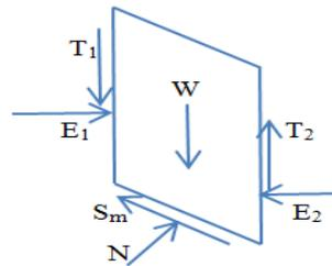
Figure 2: Forces Acting on a Slice in OM
