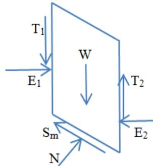
Figure 4: Forces Acting on a Slice in JSM
