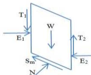
Figure 5: Forces Acting on a Slice in M-PM
