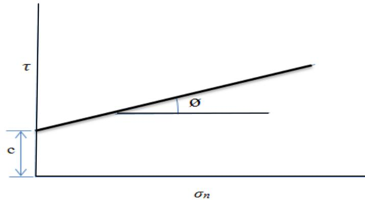
Figure 6: Graphical Representation of Coulomb Shear Strength Equation
