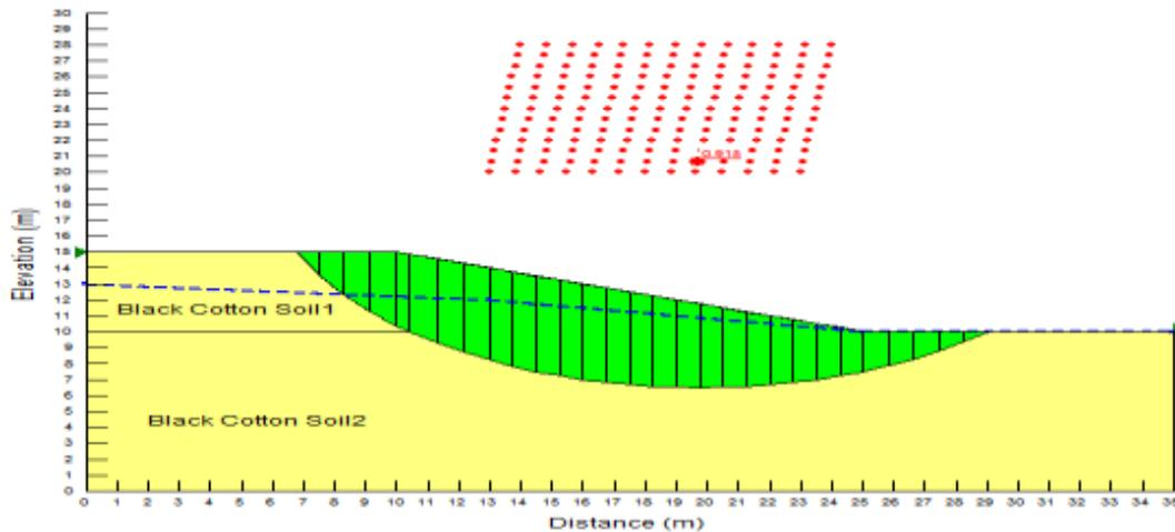
Figure 12a: Graphical View of the Computed Detail for Partially Saturated Slope
