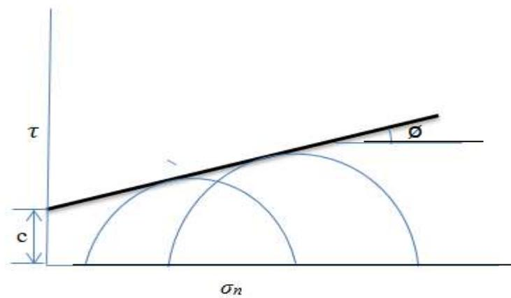
Figure 7: Mohr- Coulomb failure envelop
