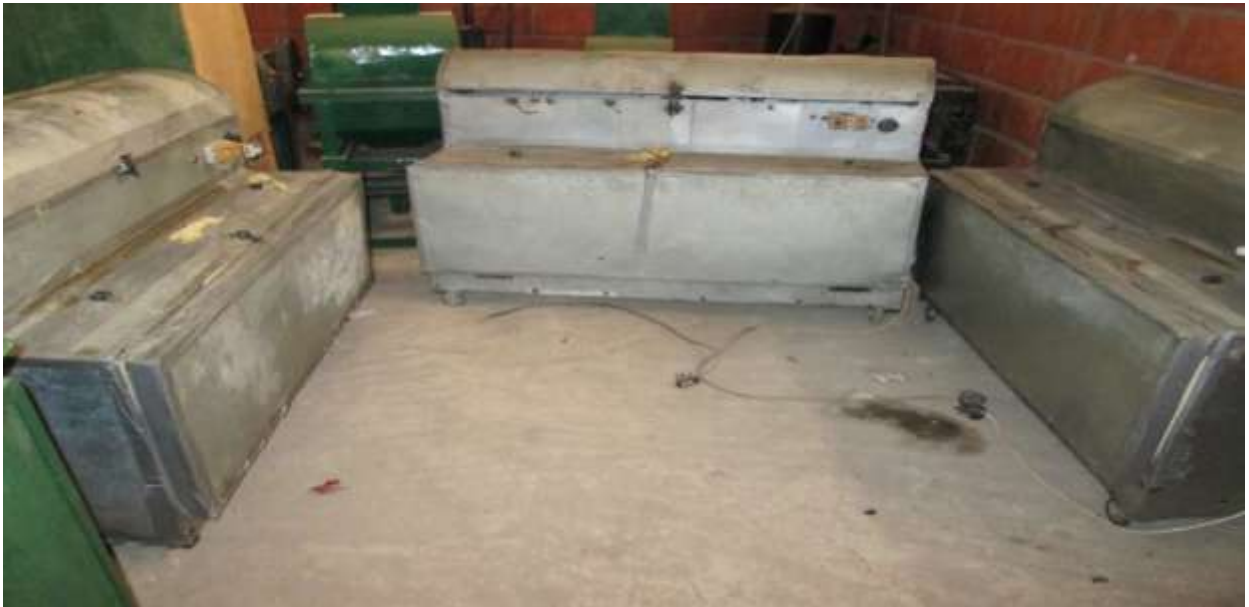
Plate 1: Three Galvanized Aluminium Cabinets for Determining the Effect of Temperature and Relative humidity on Onion Storage
