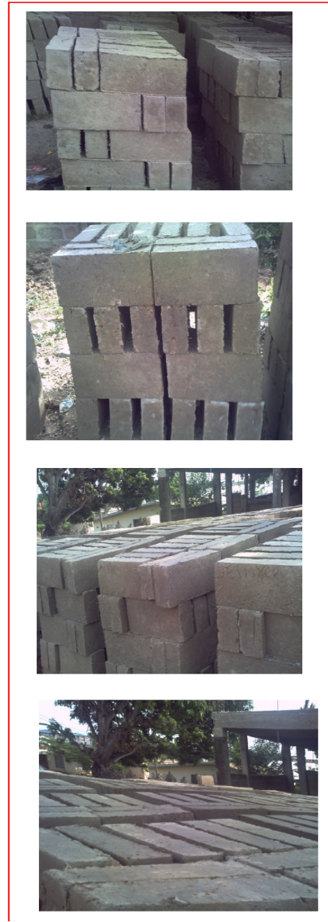
Fig. 7 b: Recommended Ways of Storing Blocks
