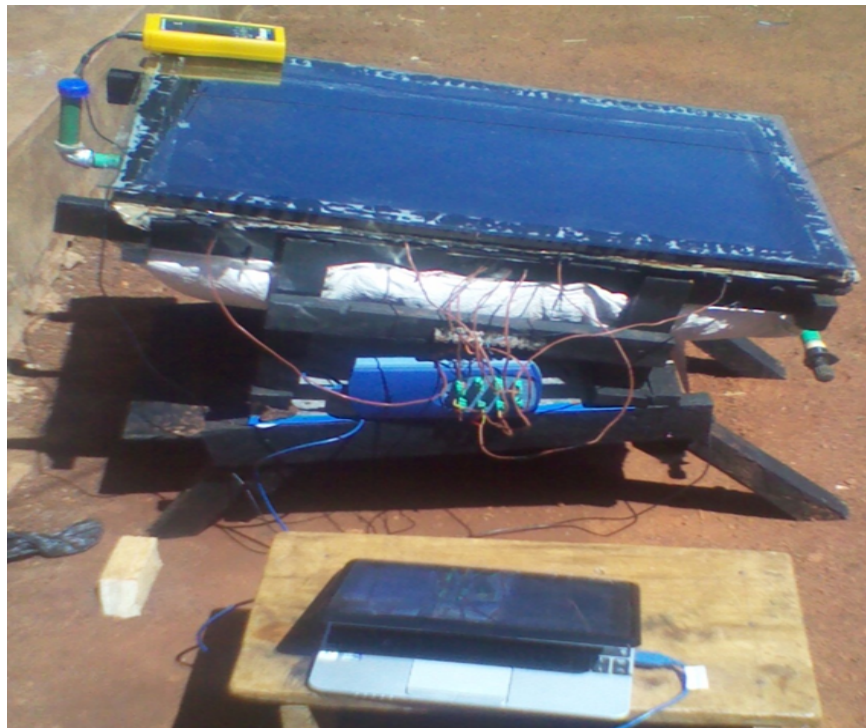
Figure 1: The Test Prototype Connected to Data Logging Equipment
