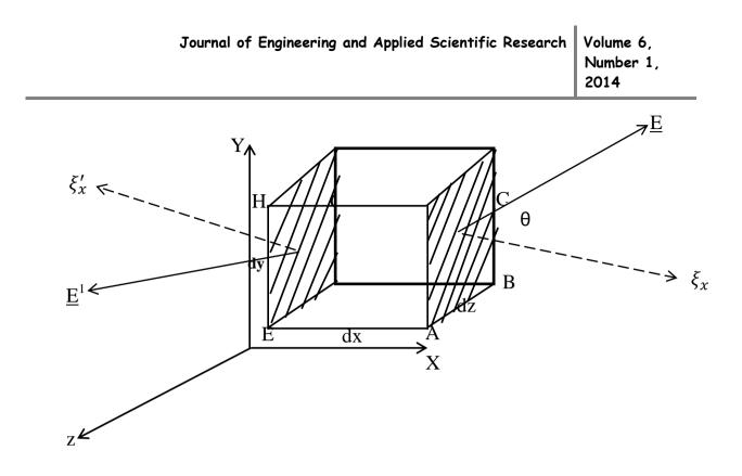
Figure 1.1. Representation of Gauss's Law of Electric Field
