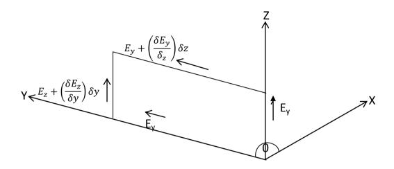
Figure 2.1. Rectangular Loop in the y - z Plane for Evaluating the Line Integral E, dl.
