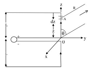
Fig 3.2a. A Linear Dipole Antenna of Length 2L
