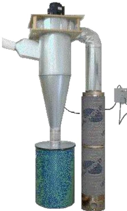
Fig 1 cyclone separator.
