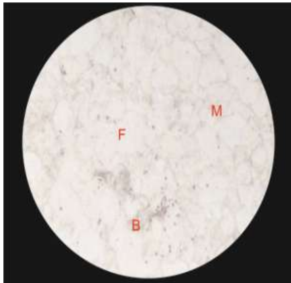
Plate 6: M= Muscovite, F=Feldspar, B=Biotite (Biotite Granite)
